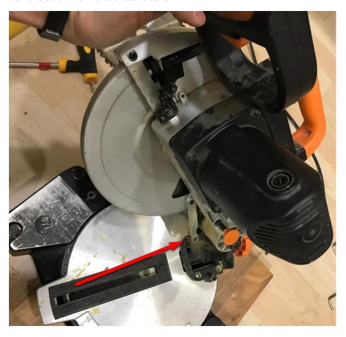
Lift saw up. Lift safe cover when needed to expose blade.
