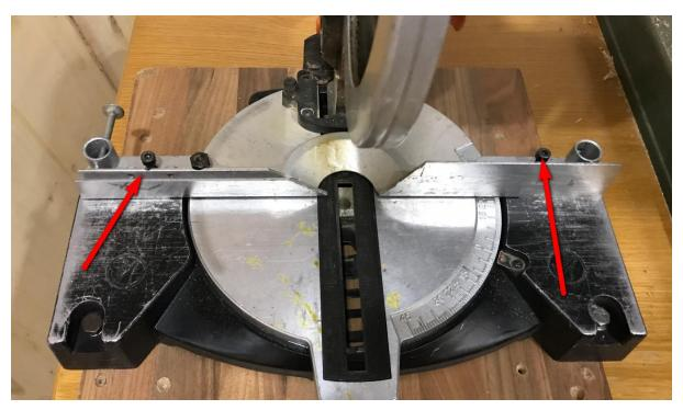
Ensure that holder is correctly positioned in the right angle.
