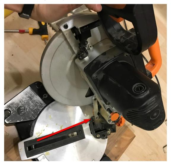
Ensure that the rubber is still on the holder holding on the position depicted on the below picture.
