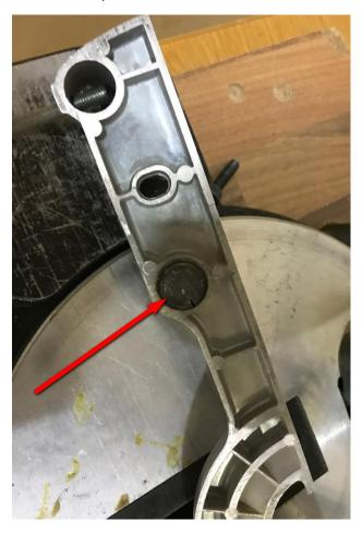
Remove bolt which holds the safe cover.
