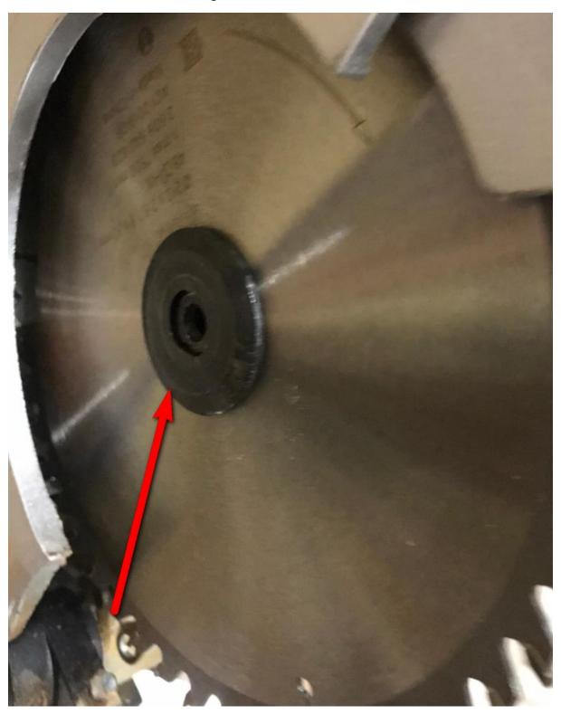
The holding bolt should go out easily. If you can't unscrew easily, please use WD40. Wait a while and try again. **Unscrewing is clockwise**!
