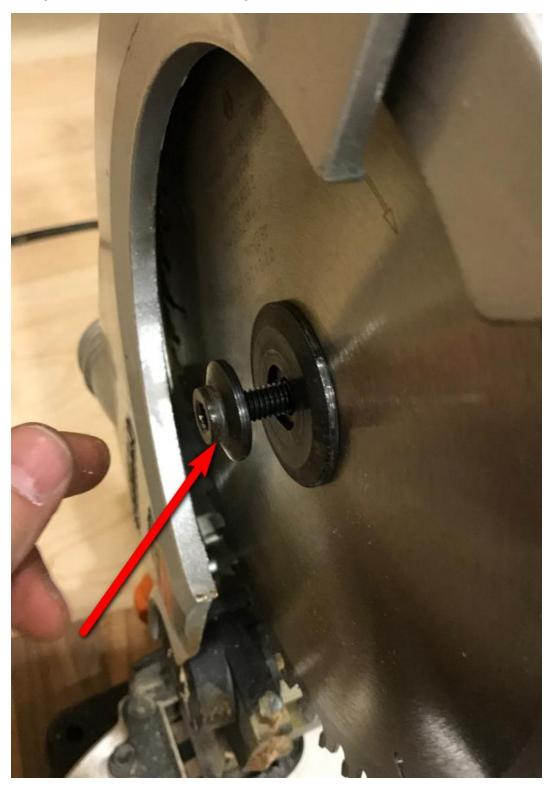
Test by hand manually that the blade turns freely.
