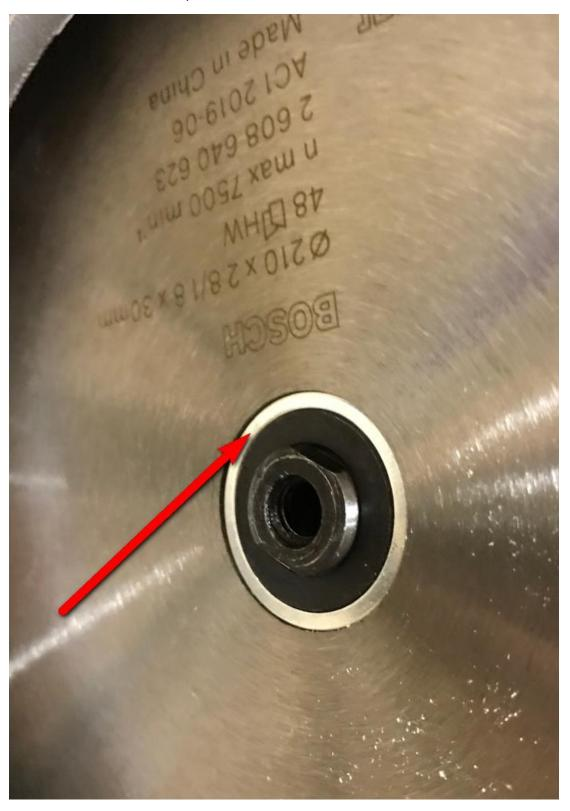
Screw back the bolt which holds the blade. The bolt has to be fastened firmly! Please use reasonable strong force to screw the bolt. **Screwing is anti-clockwise.**
