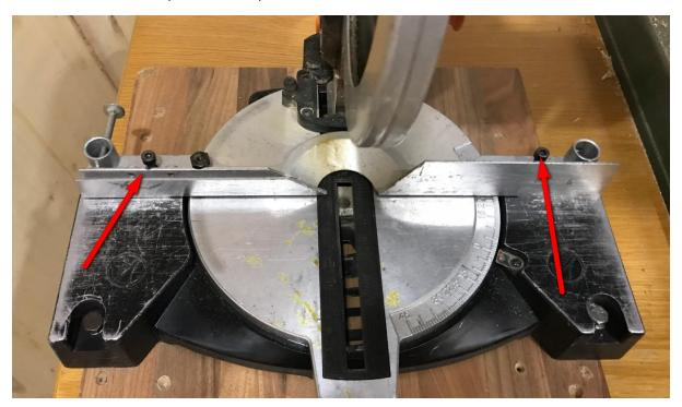
Please ensure that you don't lost rubber for securing turning plate. The rubber poistion is depicted on the below picture.
