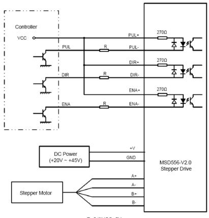
R=0 if VCC=5V; R=1K (Power > 0.125W) if VCC=12V; R=2K (Power > 0.125W) if VCC=24V; R must be connected to control signal terminal.
